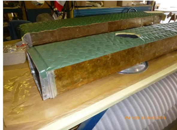
*One of the refurbished heater duct sections with a new fabric headliner secured to the top. The sides are covered with mica insulation that was removed, cleaned and reattached after repairs to the metal duct. These will be installed in the main cabin.*
