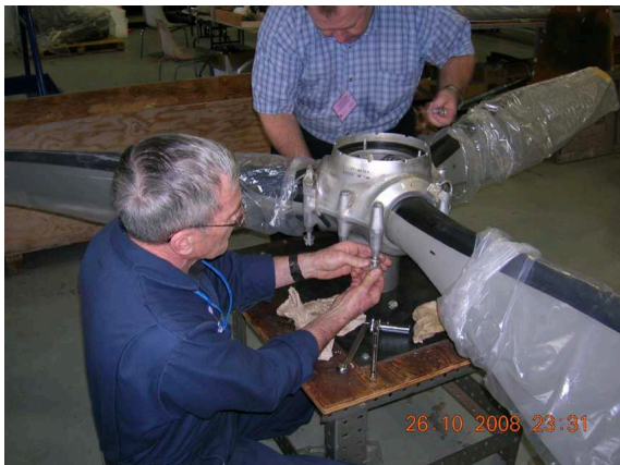
Mike Hope and Bruce Gemmill assembled Prop 1 ready to install on Engine 1 October 26, 2008.
