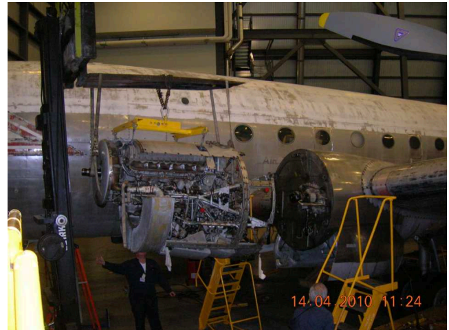
Engine 2 removed April 14, 2010.
