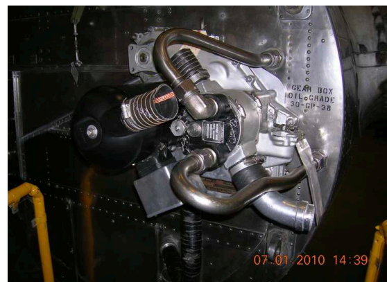
Firewall ready, auxiliary gearbox installed Jan 7, 2010.
