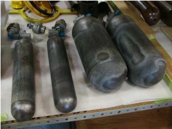
Figure 9: Fire suppressant cylinders ready for painting
