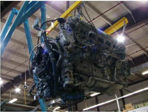
Figure 2: Disassembly underway – intake and supercharger removed
