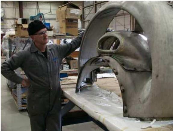
Figure 4: Murray Beaulieu prepares to restore the lower front intake cowling: replace zeus fasteners, remove dents, repair corroded sections, polish...
