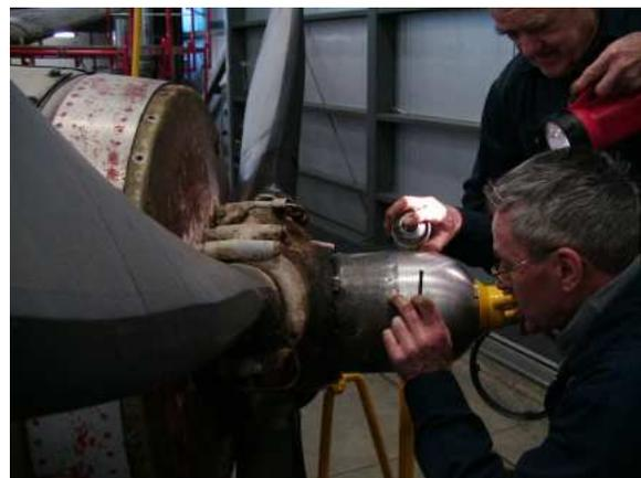
Figure 8: Number2 prop removal, Ted Devey holds light, Bruce Gemmill applies the liquid wrench.
