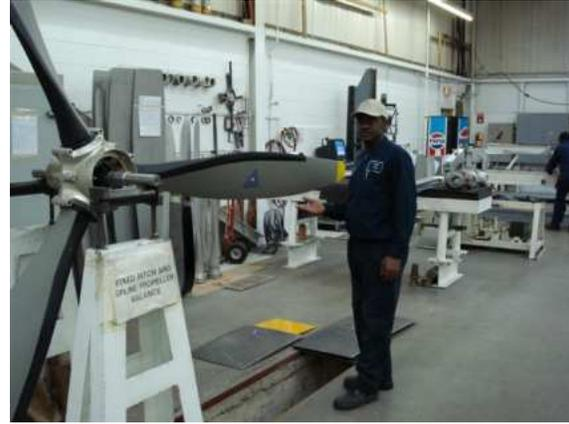
Figure 2: Hope Aero Technician Errol Brown with complete propeller mounted on the balance stand. (Photo courtesy of Hope Aero)
