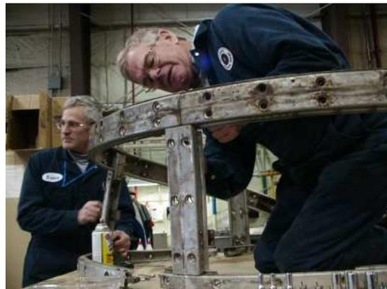
Figure 5: Cowling ring dis-assembly
