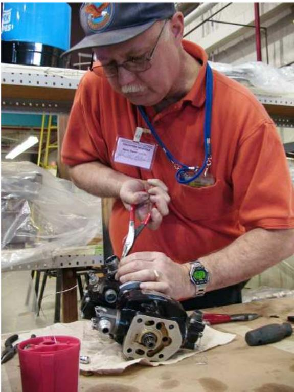
Figure 2: Lockwiring by Gary Dupont
