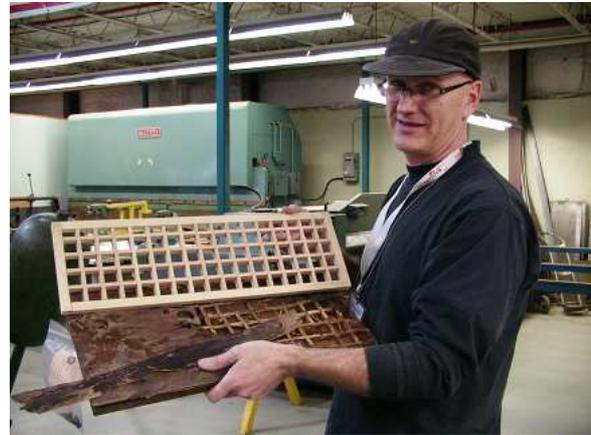
Figure 4.0.2: Murray Beaulua is building replacement sections for the cockpit floor
