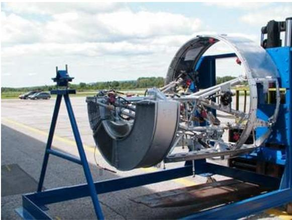
Figure 1.0.2: Power pack with connectors ready for remounting of the engine
