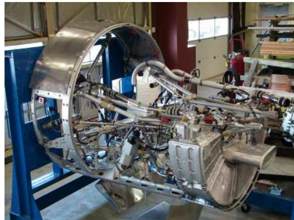
Figure 3.0.1: Engine Mounting Frame
