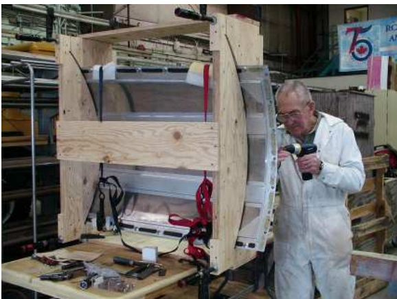
Figure 5: Ted Slack rebuilding engine panel
