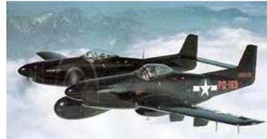
The F82F was powered by Packard Merlin engines
