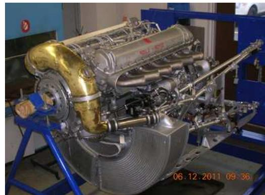
Merlin Engine Nr.2 being re-assembled in the engine shop.
