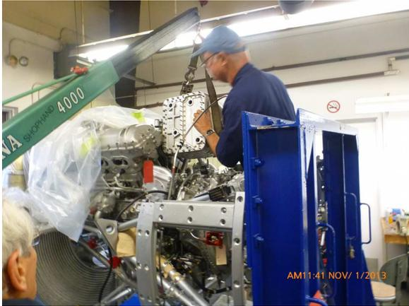
*Garry installing the intercooler on engine 3.*
