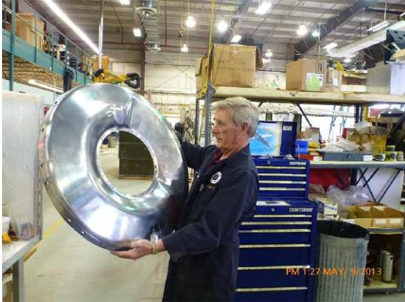
*John Thibert with the propeller cowling for engine nr 3.*
